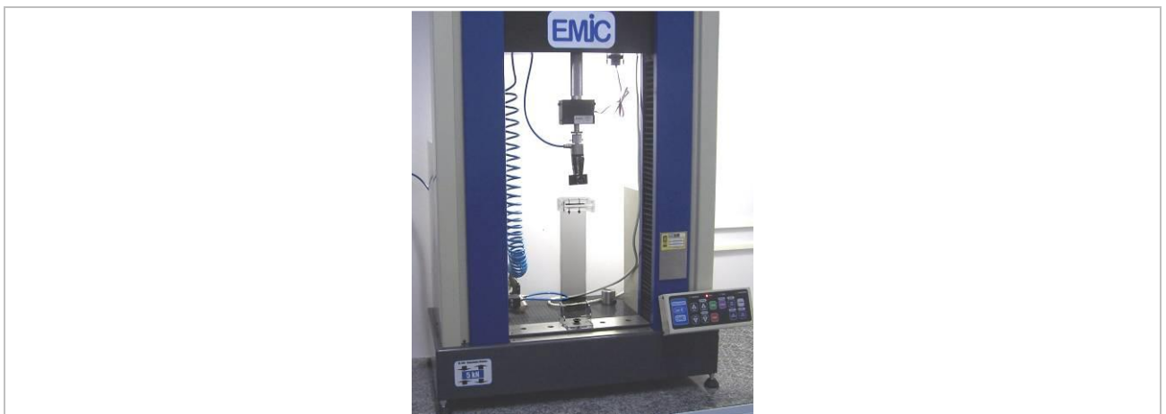
Figure 1. EMIC DL - 500 test device with comb holder.
